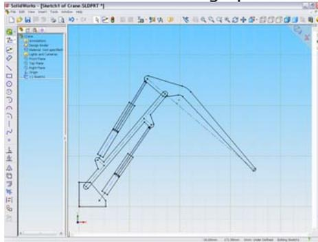
*Blocks in the sketcher are used to layout mechanisms in 2D and convert them into an assembly with parts based on each block.*
