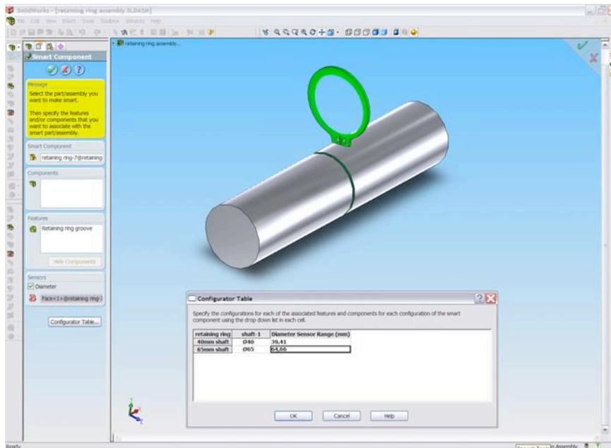
Smart Components speed design by automatically sizing a part based on the diameter of a mating part.
