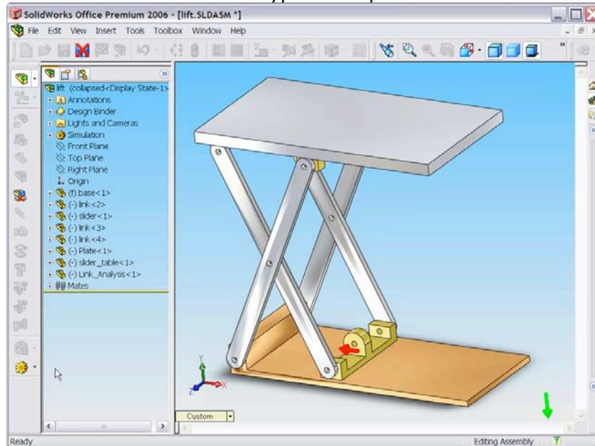
*Physical Simulation allows designers to insert motors and gravity in order to simulation how assemblies operate in real life.*
