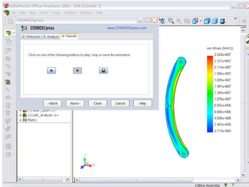
*With the problem setup automatically using the forces from how the assembly moves, designers using COSMOSXpress can now see if the design of the link arm is sufficient.*
