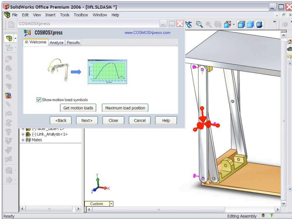
*The forces from physical simulation can then be transferred to COSMOSXpress to set up the boundary conditions for a structural analysis of the link arm of the lift assembly. This automation reduces the need for users to worry about how to correctly set up the structural analysis.*
