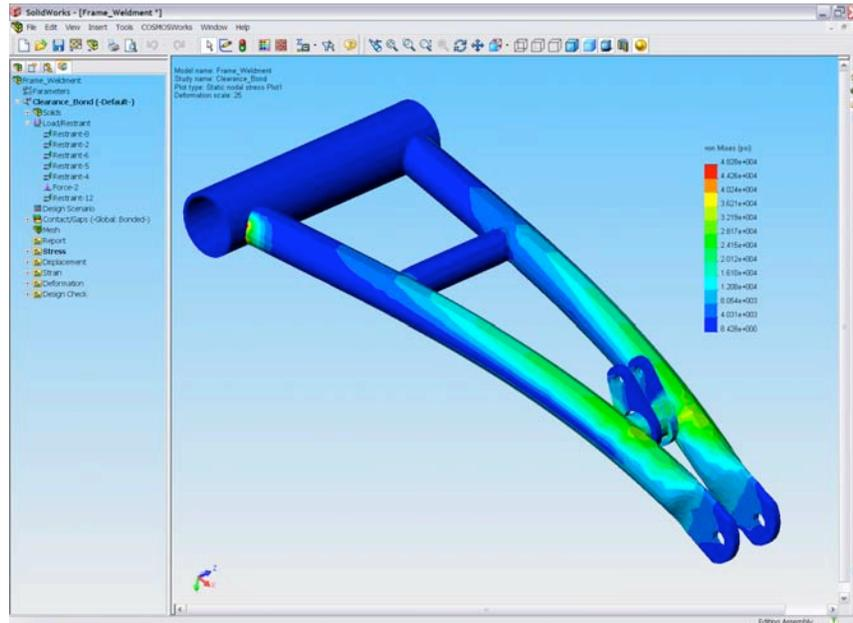
*Note the gap where the connectors join the lower support*
