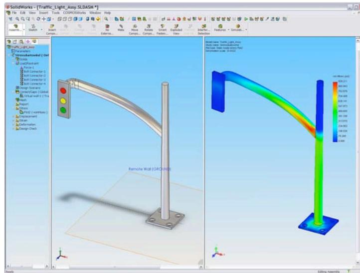
*Bolt behavior of the traffic light post is modeled using the grounded bolt connector in COSMOSWorks 2006*
