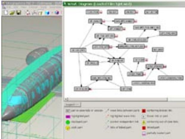
The image above displays a WAVE diagram that expands the detail of the previous image; it can show as much or as little detail as desired. This diagram shows two levels.
