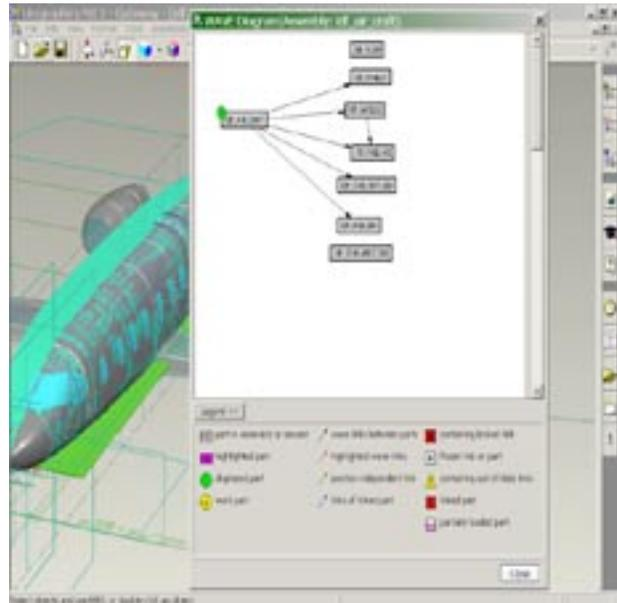
*The image above depicts a simple first-level WAVE diagram for a small business jet. Only a portion of the control diagram is displayed. Note the clarity of the controlling parameters and their notation.*
