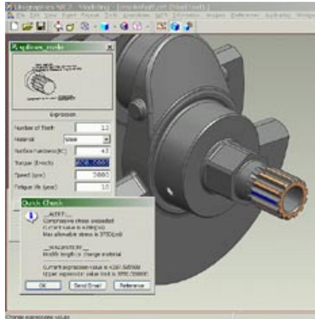
*In the image above a pre-planned NX Quick Check shows that the user has violated a simple analysis check on the allowed compression value. Performing this check during the assembly process ensures product validity at design time rather than later - a better technique.*
