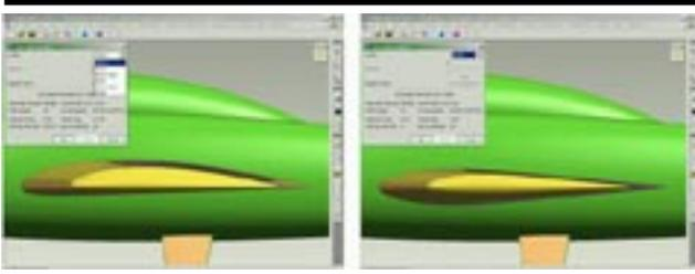
Major topological swapping of subsystems like the replacement of this tail assembly or the replacement of the landing gear from a tricycle configuration to a tail-dragger can also be performed. Also, an optimization loop for positioning the landing gear relative to the center of mass of the plane (to which the landing gear contributes, of course) is included in the system model.
