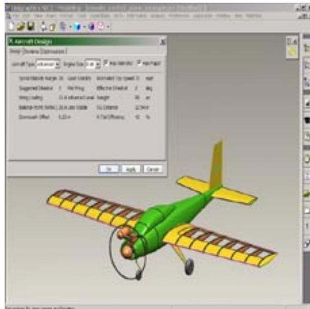
*The above image shows a custom designed user dialog built with NX Knowledge Fusion tools to improve usage of a pre-defined KF function for “model airplane design.”*
