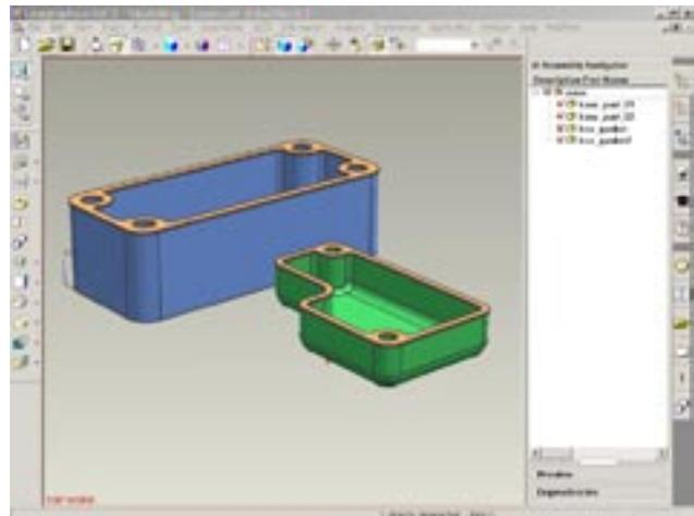
The image above shows completed box assemblies, each with their intelligent gaskets built by linking the gasket part to different faces.
