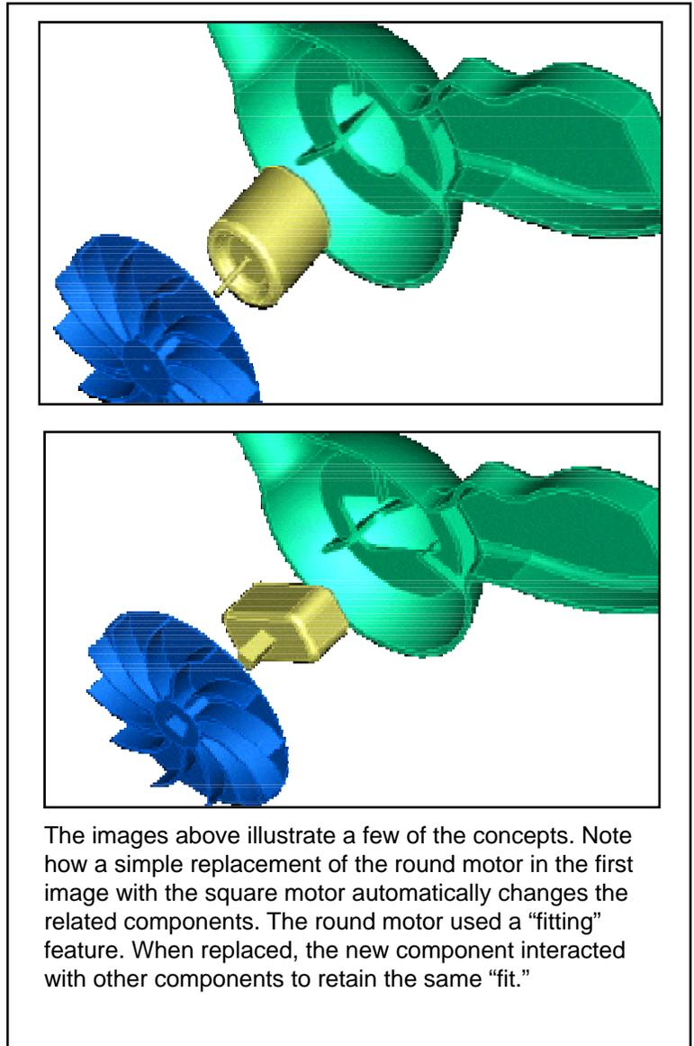
the resulting geometry" message or "missing constraints." *Functional modeling avoids this paradox by encapsulating within its features, the intelligence about how to interact with other features.*
