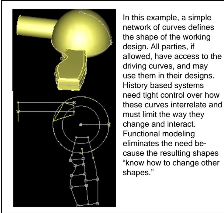
In this example, a simple network of curves defines the shape of the working design. All parties, if allowed, have access to the driving curves, and may use them in their designs. History based systems need tight control over how these curves interrelate and must limit the way they change and interact. Functional modeling eliminates the need because the resulting shapes "know how to change other shapes."
